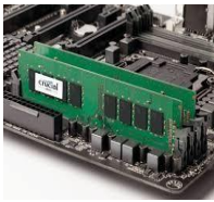
RAM chips fitted in expansion slots
